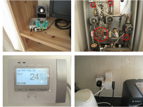
Fig. 7. Examples of home network components deployed in the prototype installation. Starting clockwise from the top left corner, they depict a UWB platform measuring occupancy, Xbees sensor monitoring the boiler operation, a Zigbee HA plug module and a Zigbee HA Thermostat.
